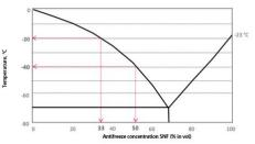
Dilutition of 50% gives an antifreeze protection up to -40°C, dilution of 33% gives protection up to -20°C. Dilution of 65% gives maximum antifreeze protection up to -69°C. Dilution bigger than 70% in water are not anti
