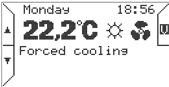
Figure 4.8 Forced summer ventilation mode
