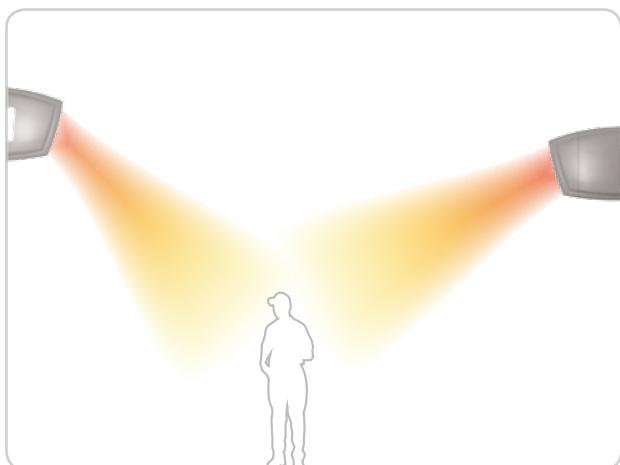
Correctly installed heaters should direct the air to the occupied zone.
