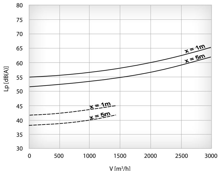
Acoustic characteristic of fan with damping roof base (HPDT, HPDTs)
