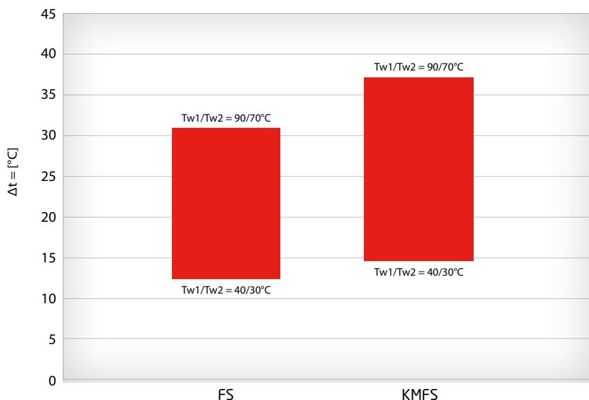
Air temperature rise at unit's maximum air flow. Inlet air temperature 0°C.
