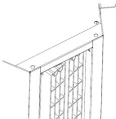
The device is equipped adjustable outlet grilles. The angle should be set manually within  $\pm 17^\circ$ . The airflow from the outlet grille should be directed as close as possible to the plane of the door opening (taking into account the conditions prevailing at the door opening).
