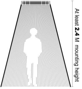
**Note**: Indoor or well-protected environments will generally exceed average coverage areas. Heaters can provide less than average coverage in extremely cold/windy conditions.
