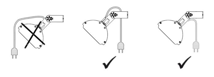
Attention:Digital display position should be on left for correct installation direction
