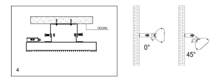
The heater must be installed at least 2.4 M above the floor Attention: cable should not passing thought the heater
