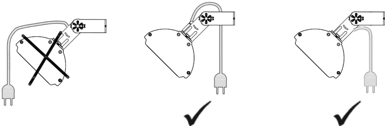
**Attention: Digital display position should be on left for correct installation direction**
