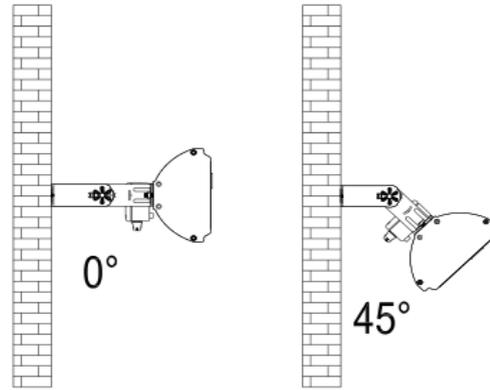
**The heater must be installed at least 2.4 M above the floor**
