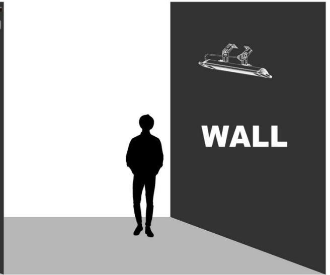
**Note:** Heater should be wall or ceiling mounted under well protected environments, at least keep 3feet (0.9m) away from any combustibile objects.
