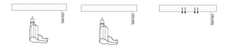
A wall mounting bracket is provide with the heater which has been specifically designed to allow this product to be fitted to a wall or ceiling before drilling the holders for the wall/ceiling is solid and that there are no hidden water pipes or electric wires. The heater must be installed no less than 16" form side walls and no less than 6" off the floor.
