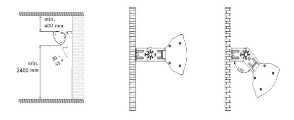
The heater must be installed at least 2.4M above the floor Attention: cable should not passing thought the heater
