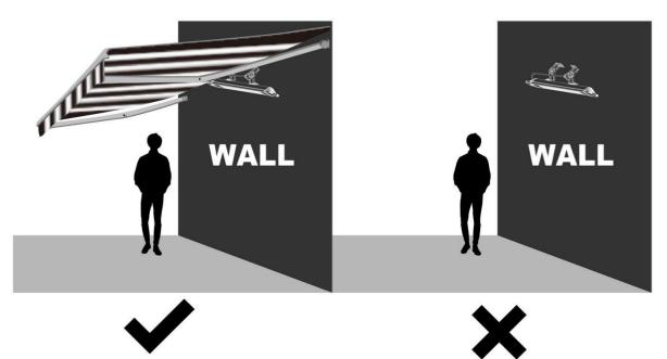
**Note**: Heater should be wall or ceiling mounted under well protected environments, at least keep 3feet (0.9m) away from any combusitble objects.
