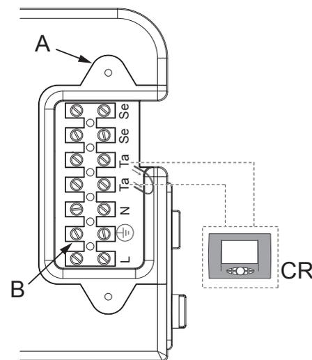
A Plate on the boiler electrical panel
