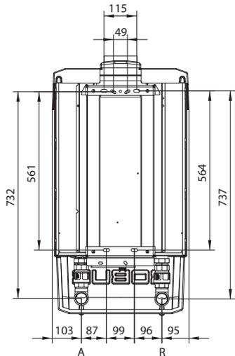
A Outlet  $\varnothing 1 \frac{1}{4}$ " M      R Inlet  $\varnothing 1 \frac{1}{4}$ " M
