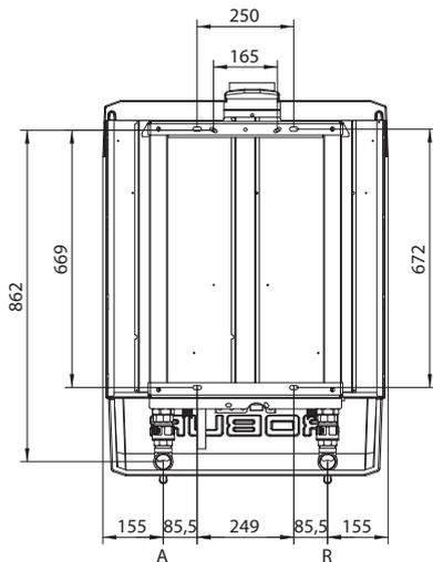
A Outlet  $\varnothing 1 \frac{1}{4}$ " M      R Inlet  $\varnothing 1 \frac{1}{4}$ " M
