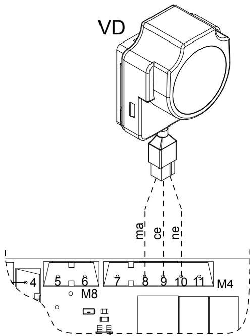
VD Buffer tank diverter valve for DHW charging
