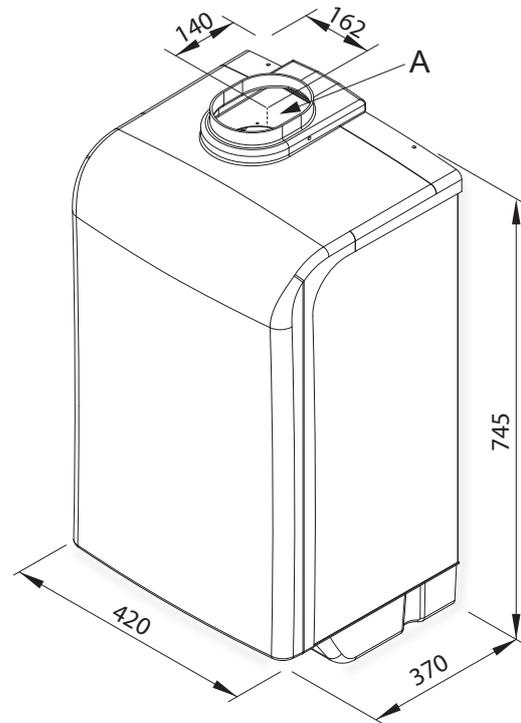
A Flue gas outlet  $\varnothing$  80 mm
