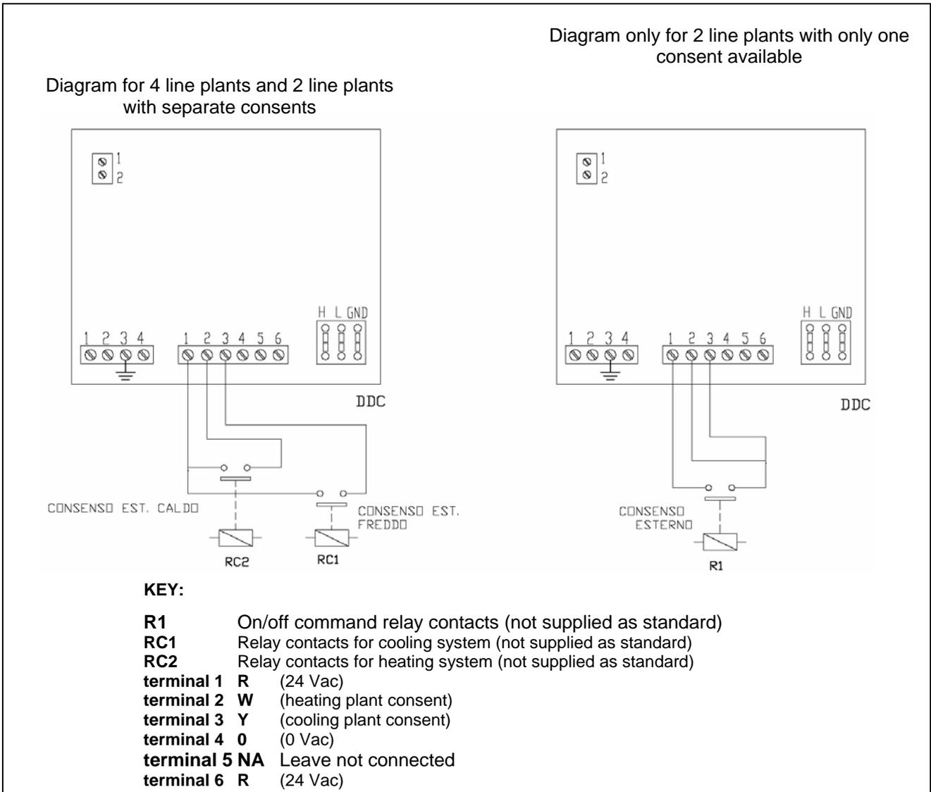
**Figure 26** – EXAMPLE OF EXTERNAL CONTROL PLANT CONNECTIONS FOR RYW<sub>m</sub> MODE
