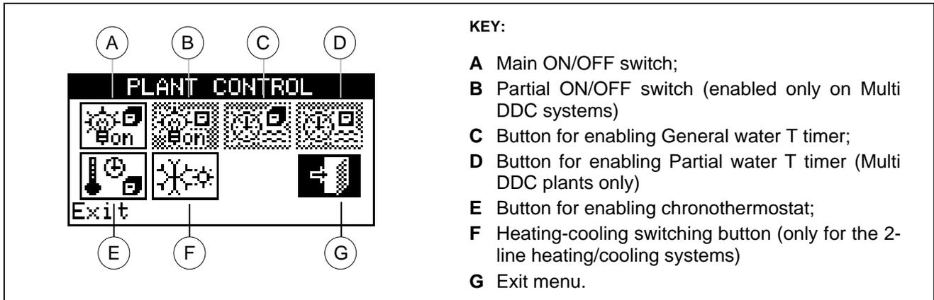
Figure 3 – EXAMPLE OF COOLING/HEATING PLANT CONTROL SCREEN
