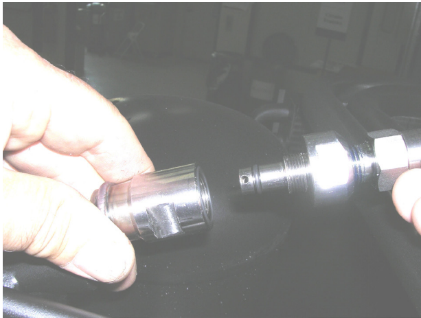
Figure 9.7 Removal of safety valve mobile part - Removal of safety valve
