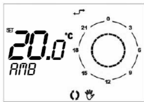
Figure 6.7 Forced automatic operation
