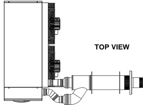
**ATTENTION:** The above mentioned lengths are intended for installations in which the air and exhaust ducts are on linear paths as represented in the figure. If this is not the case, you must calculate the pressure loss (see SAMPLE CALCULATION).
