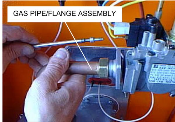
Figure 36 – Gas pipe/flange assembly
