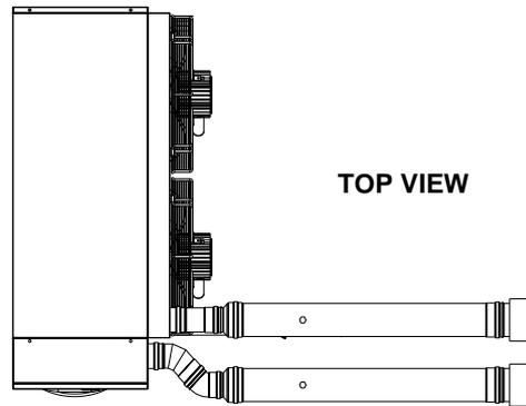
**ATTENTION:** The above mentioned lengths are intended for installations in which the air and exhaust ducts are on linear paths as represented in the figure. If this is not the case, you must calculate the pressure loss (see SAMPLE CALCULATION).
