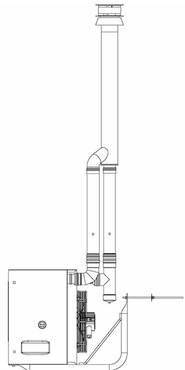
**ATTENTION:** The above mentioned lengths are intended for installations in which the air and exhaust ducts are on linear paths as represented in the figure. If this is not the case, you must calculate the pressure loss (see SAMPLE CALCULATION).
