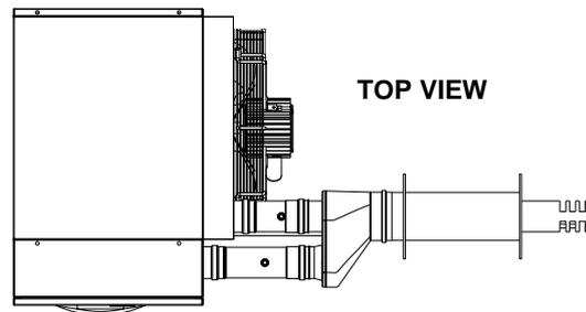
**ATTENTION:** The above mentioned lengths are intended for installations in which the air and exhaust ducts are on linear paths as represented in the figure. If this is not the case, you must calculate the pressure loss (see SAMPLE CALCULATION).
