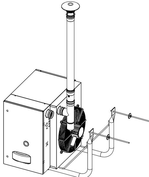
**ATTENTION:** The above mentioned lengths are intended for installations in which the air and exhaust ducts are on linear paths as represented in the figure. If this is not the case, you must calculate the pressure loss (see SAMPLE CALCULATION).
