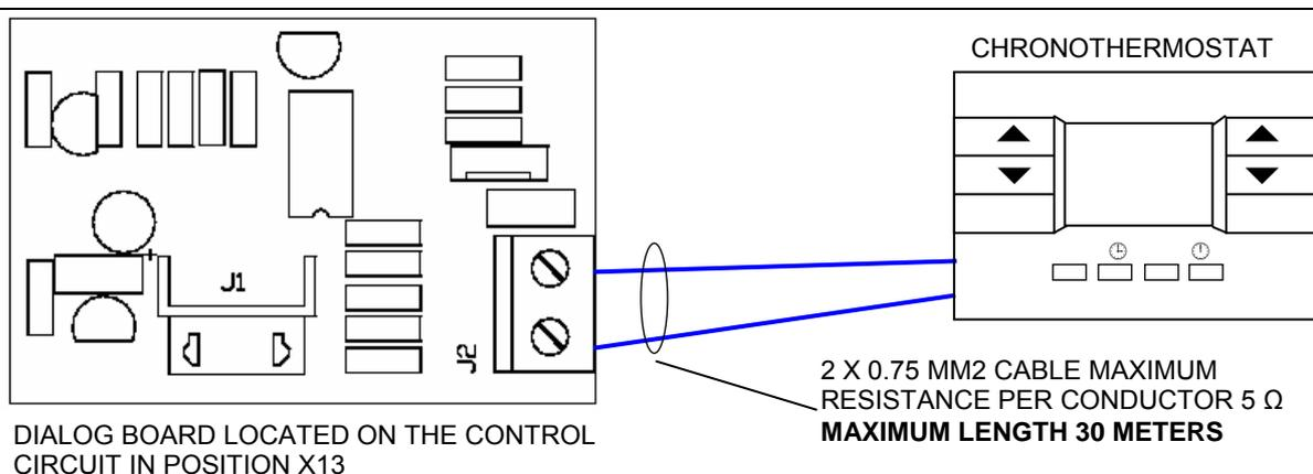
**Figure 31** – Connection of chronothermostat and dialog board
