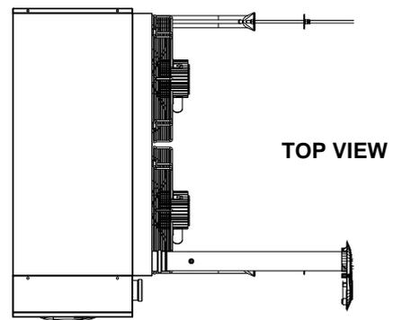
**ATTENTION:** The above mentioned lengths are intended for installations in which the air and exhaust ducts are on linear paths as represented in the figure. If this is not the case, you must calculate the pressure loss (see SAMPLE CALCULATION).
