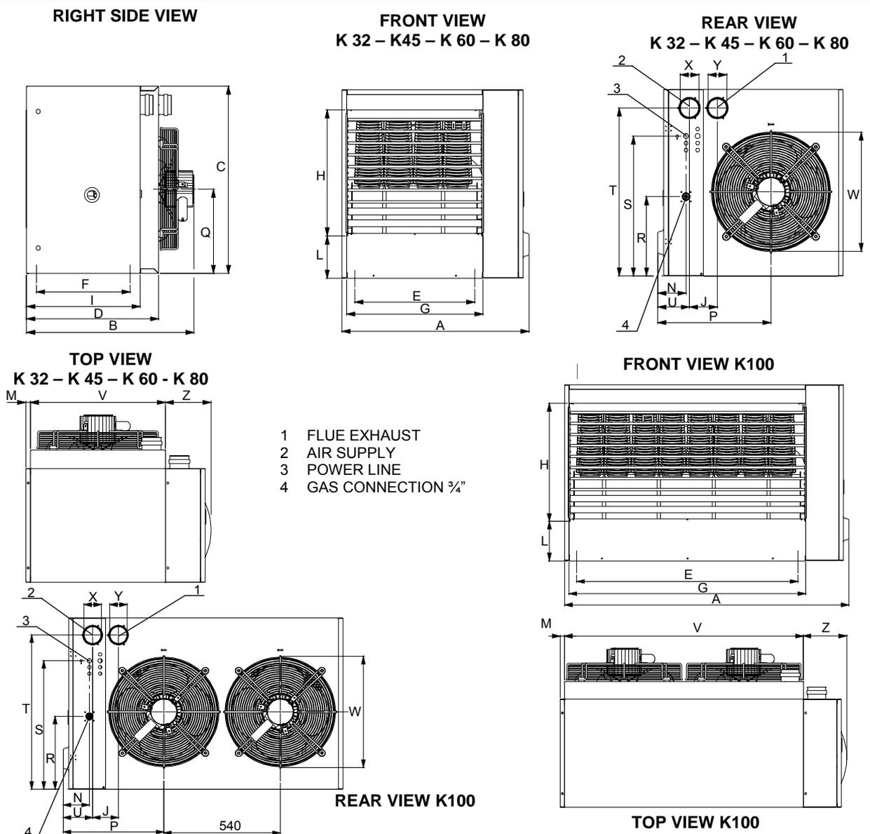
Figure 1 – Dimensions of the K series heating units
