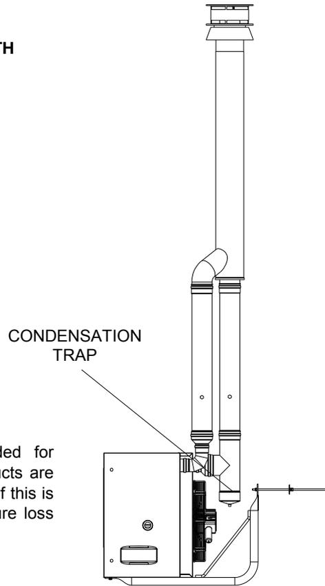
**Figure 24** – C33 coaxial roof type installation with Ø 130 ducts
