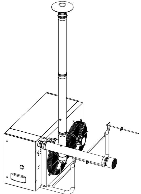
**Figure 26** – C53 type installation with Ø 110 pipes
