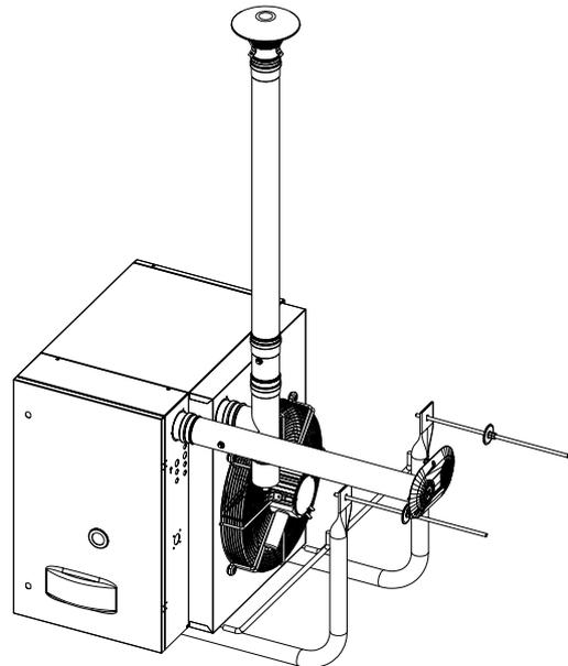
**Figure 25** – C53 type installation with Ø 80 pipes
