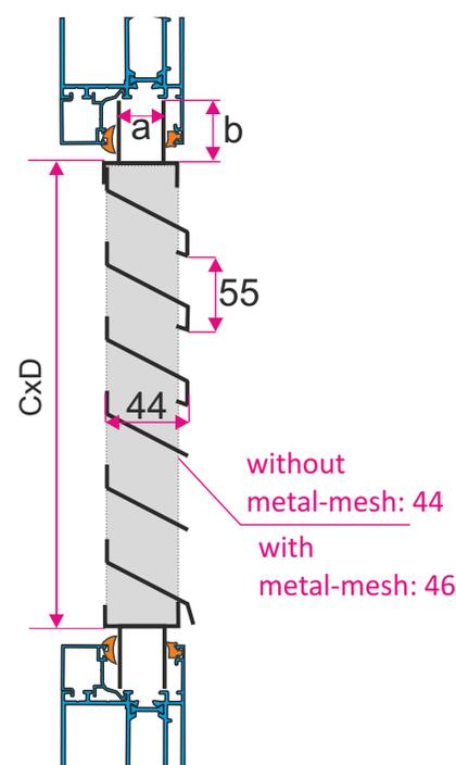
Intakes louvres for installation in a door or window profile made on order are in adapted sizes to individual customer needs.
