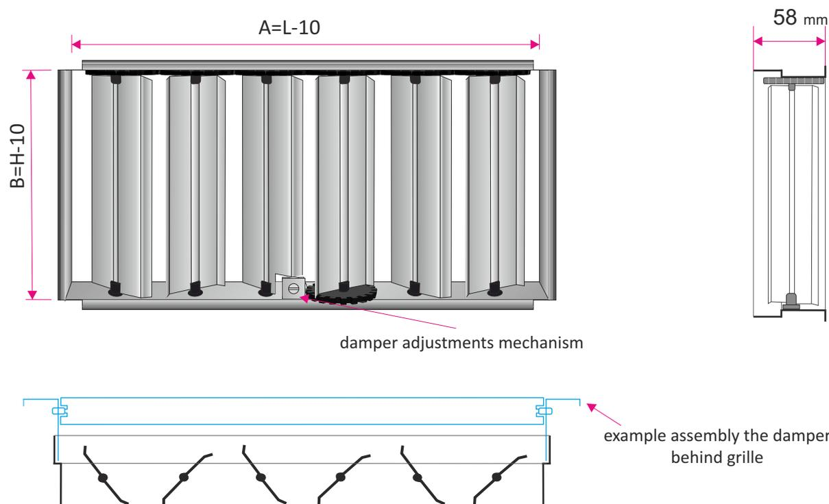
To change the damper blades first you must unlock the mechanism by gently removing the screw (turn left). Then set blades at an specified angle and block the mechanism by gentle turning the screw (right) until you feel resistance.
