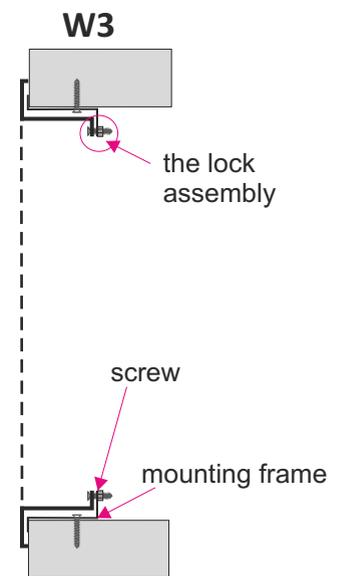
Assembling invisible by screws and lock assembly in mounting frame RM or in plenum box. Option recommended for invisible installation in the ceiling.
