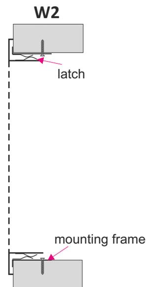
Assembling invisible by latches in grille and mounting frame RM or in plenum box.
