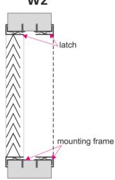
Assembling invisible by latches in grille and mounting frame RM or in plenum box.
