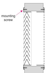
Assembling visible through screws and mounting holes in the grille frame.
