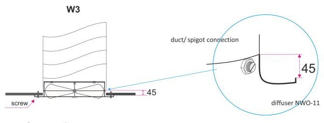
Screw mounting directly to the plate
