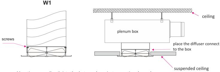
Mounting screws directly into the duct round or spigot connection plenum box.
