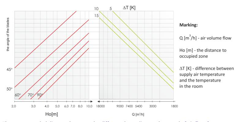
The recommended distance between the diffusers depending on the speed of air flow from the diffuser  $v_{\mbox{\tiny ef}}$  (m/s).
